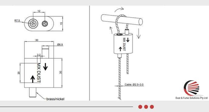
Looping Grippers are automatic adjustable cable fixers for wire rope suspension. Suitable for a variety of wire rope suspension applications.
